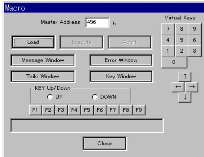
**Master Address** Specified the master address of the device in which the macro is executed.
