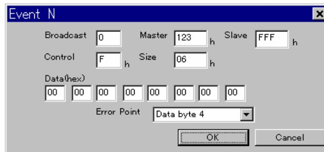
In the above setting, a timing error occurs in the fourth byte of the frame data.
