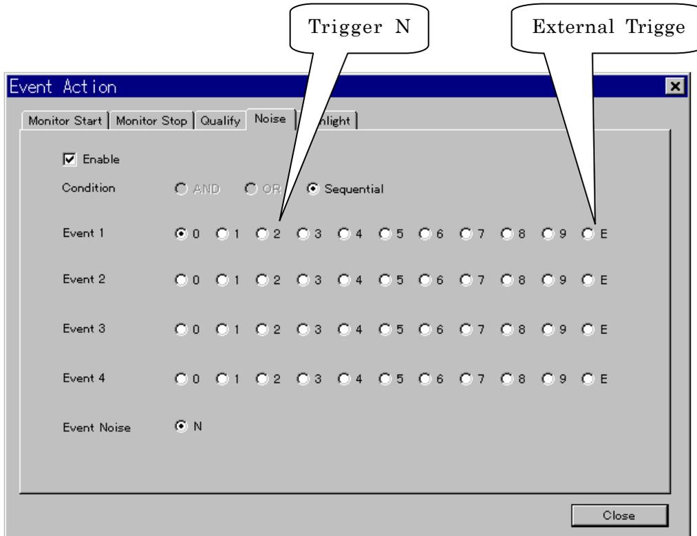
In the above trigger setting, after trigger 0 occurs, AP-IEB2 waits for detection of Even N.
