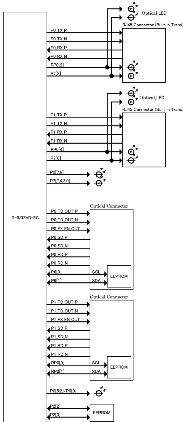
The following LEDs are mounted for monitoring Ethernet.
